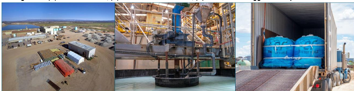
Figure 13: (A) White Mesa site, (B) Crack and leach circuit; (C) Concentrate bagged for shipment to Estonia
