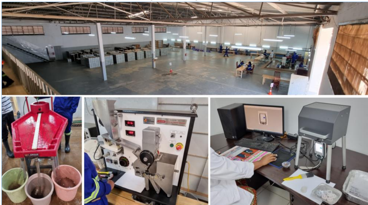
Figure 7. (A) SVM Lilonge processing lab showing (B) riffle table, (C) mag sep and (D) PXRF
