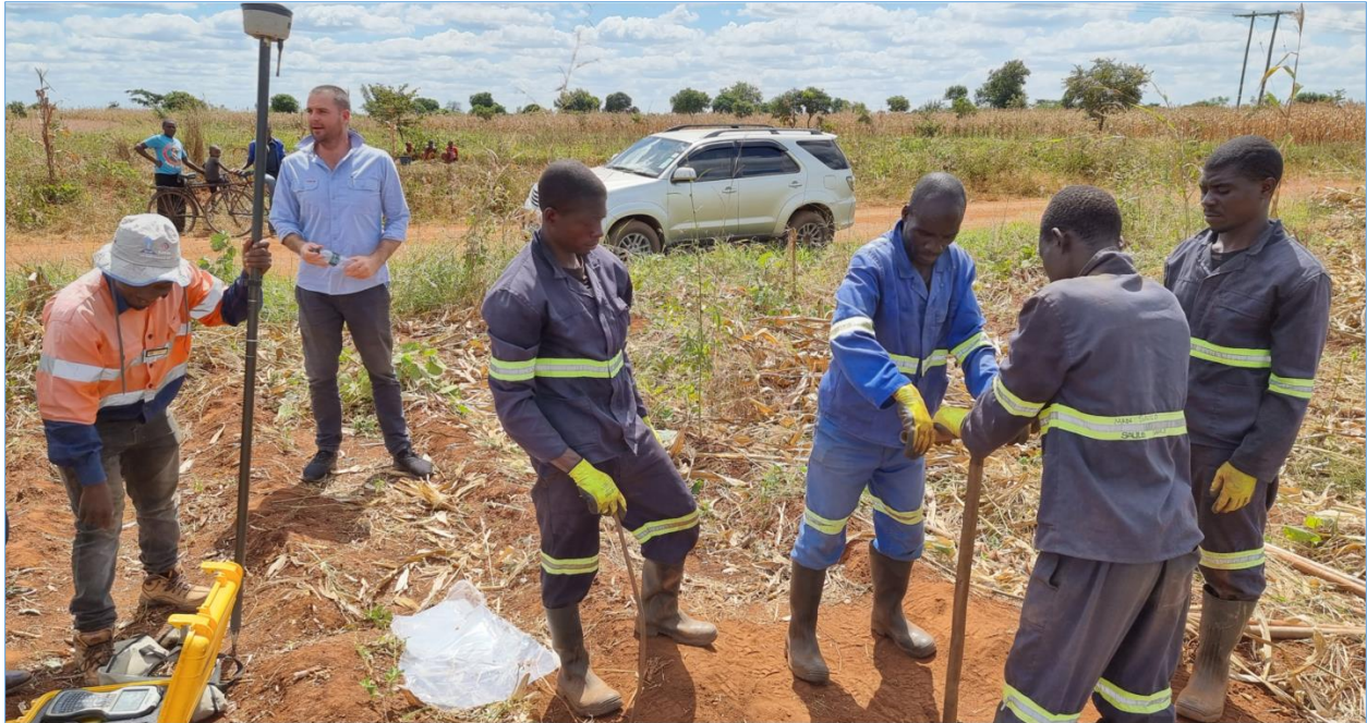
Figure 2. Hand auger drilling near power line on SVM property
