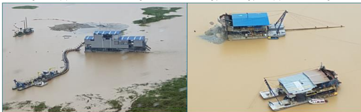
Figure 19: (A) Llanuras suction dredge and attached floating processing plant; (B) Brazilian dredges
