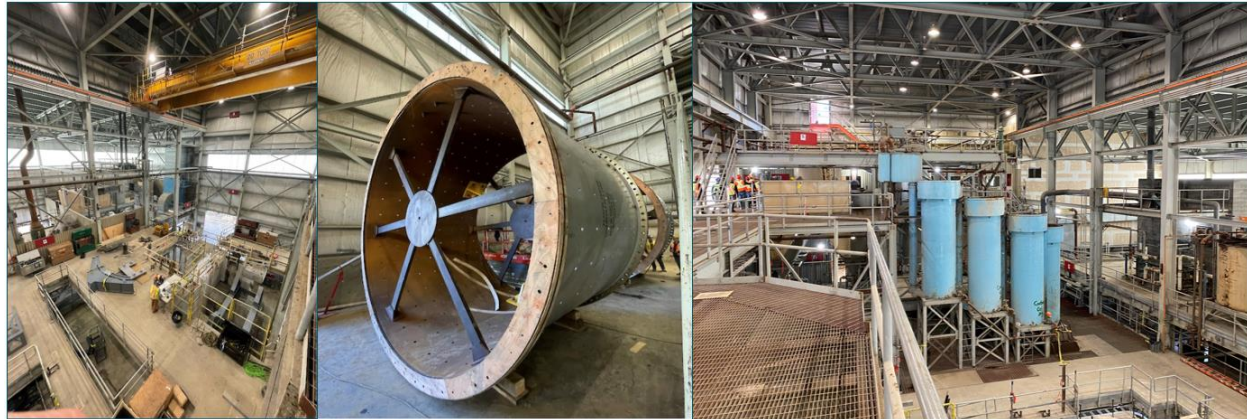
Figure 2. (A) Ball mill cradle, (B) ball mill shell and (C) interior of the processing plant including elution columns
