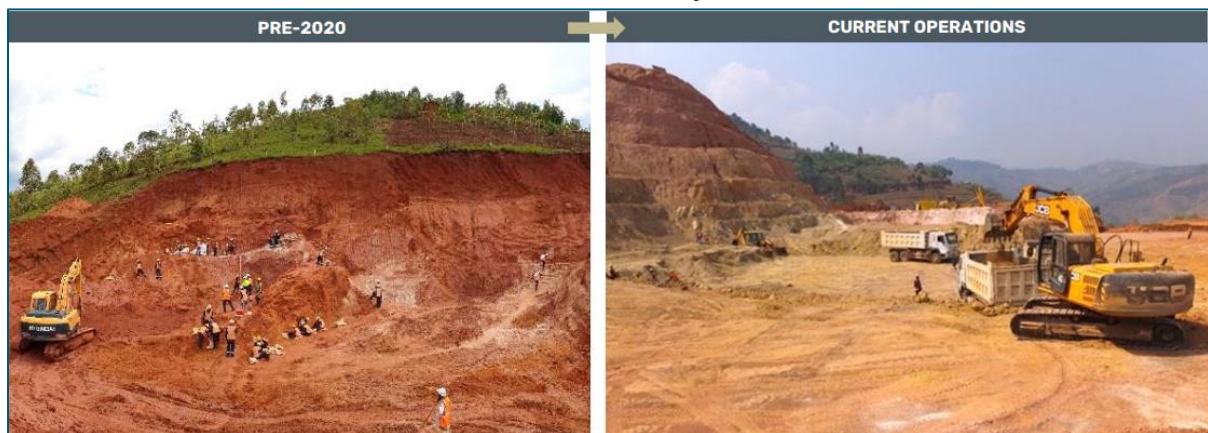
Figure 17: Mining operations at Gakara (A) Pre-2020 and (B) under current management; note the improvement in bench consistency
