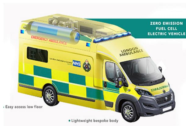
A prototype ambulance with a fuel cell powertrain is also in development. Picture credit: ULEMCo
