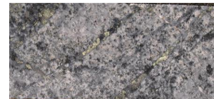
Cumbre: Near surface oxides and deeper sulfides, disseminated (l) and in sheeted veinlets (r)
