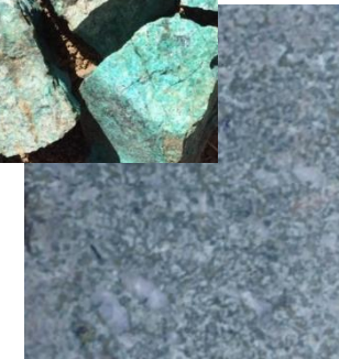
Cumbre: Near surface oxides and deeper sulfides, disseminated (l) and in sheeted veinlets (r)
